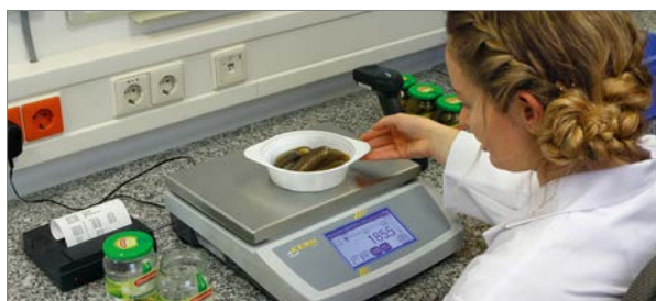
Sample testing of a pre-packaged item which is empty (destructive analysis)
